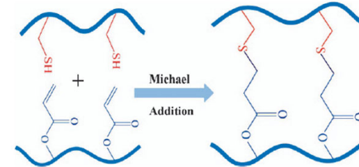
Figure 6. Schematic illustration of injectable hydrogels prepared by the Michael addition cross-linking method.
