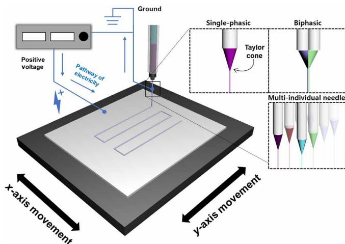
**Fig. 1. Schematic diagram of the CREW system.** The CREW system for fabrication of a fiber-based scaffold using the moving stage. The positive voltages are applied to the conductive collector. The blue lines represent pathway of electricity.
