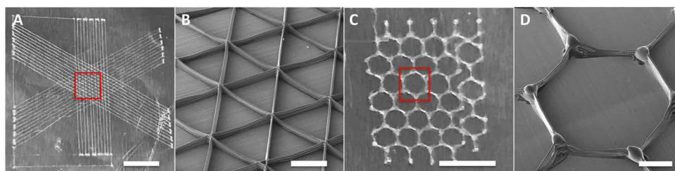
**Fig. 3. 3D printed patterns.** Digital images of 3D printed structures prepared by the CREW system representing (A) a triangular structure and (C) honeycomb. (B and D) SEM of selected parts of these 3D printed structures. Scale bars, 500  $\mu\text{m}$ .
