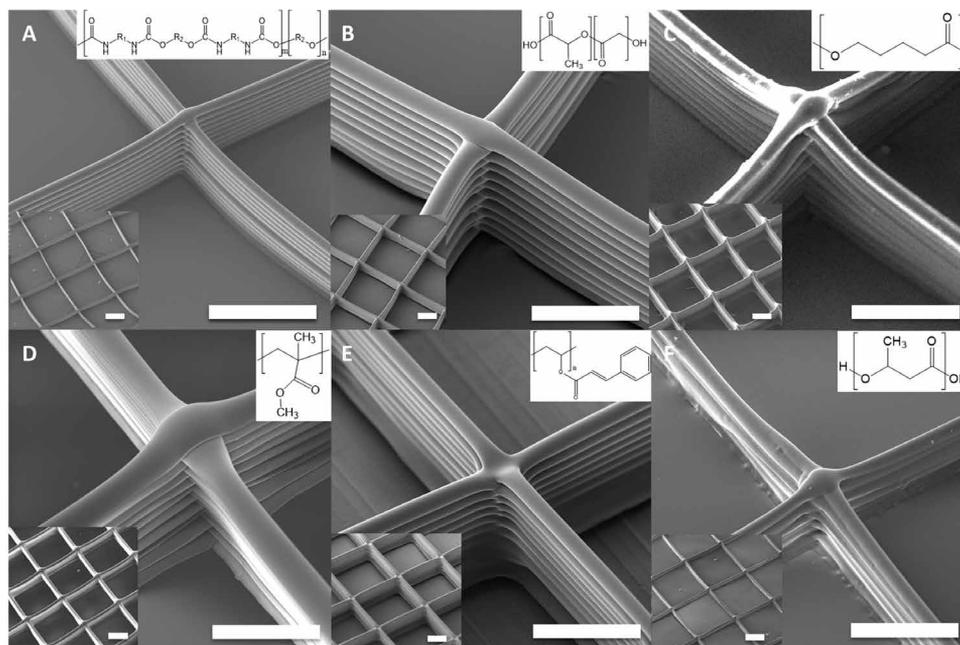
**Fig. 4. Material diversity.** SEM images of scaffolds prepared using various polymer materials by the CREW system. (A) TPU, (B) PLGA, (C) PCL, (D) PMMA, (E) PVCi, and (F) PHB were used as polymer materials, and the THF/DMF pair was used for (A) to (E) as solvent to prepare the polymer solutions, and the TFE/chloroform pair was used for (F). Scale bars, 200  $\mu\text{m}$ .
