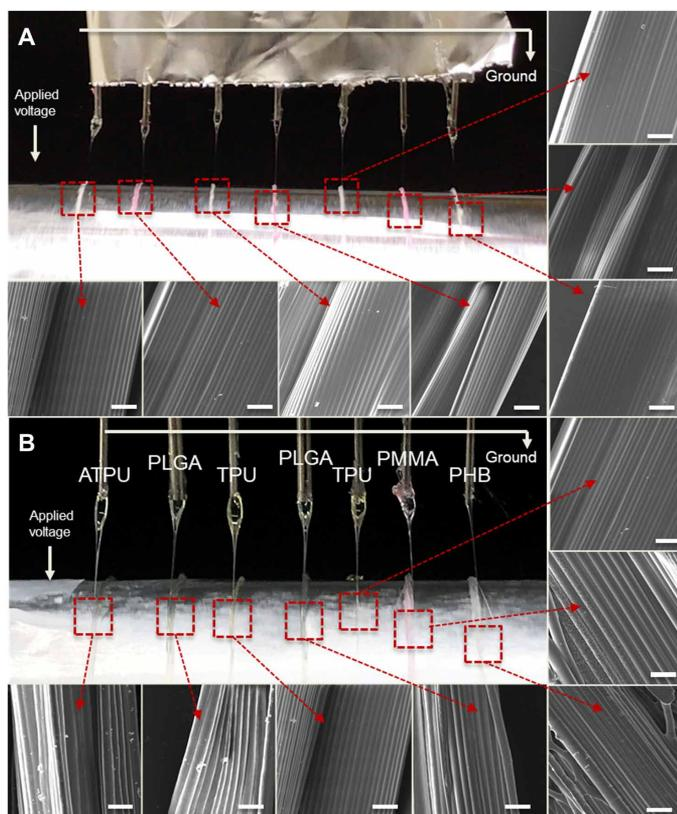
**Fig. 7. Parallelized production.** Digital images of the Taylor cones of seven polymer jets and SEM images of obtained microfiber bundles using seven needles in parallel (A) with TPU in the THF/DMF mixture with red and green dyes and (B) with various polymer materials such as the ATPU, PLGA, TPU, and PMMA in the THF/DMF mixture, and PHB in the chloroform/DMF mixture. Scale bars, 100  $\mu\text{m}$ . (Photo credit: Seongjun Moon, Chungnam National University.)
