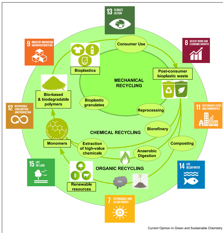
Schematic representation of recycling strategies for sustainable management of bioplastics and contribution towards SDGs.
